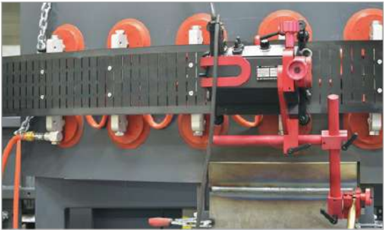
Flexible trackway length 1.88 m (6.1 ft). Minimum curvature radius of 1.25 m (4.1 ft) PRW-0466-71-00-00-0
