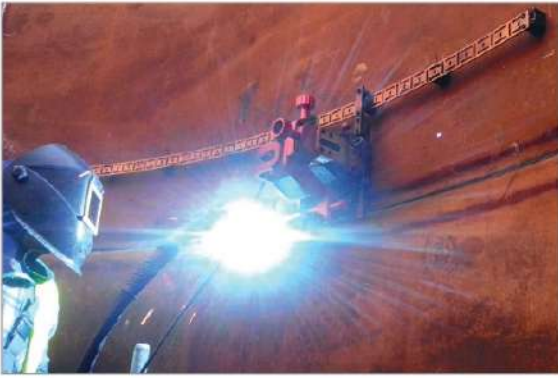
Flexible track length 185 cm (6ft) 1pc Minimum curvature radius of 1.0 m (3.3 ft) PRW-0466-50-01-01-0
