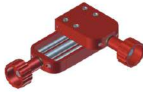
ZSP-0466-46-00-00-1 Extended cross-slide 0-76 mm (0-3") up-down, 0-35 mm (0-1.38") left-right
