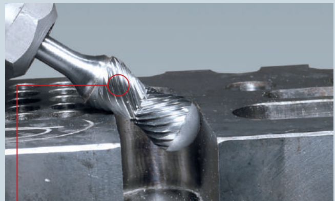
Außenfase in SKM Form External chamfer with SKM shape
